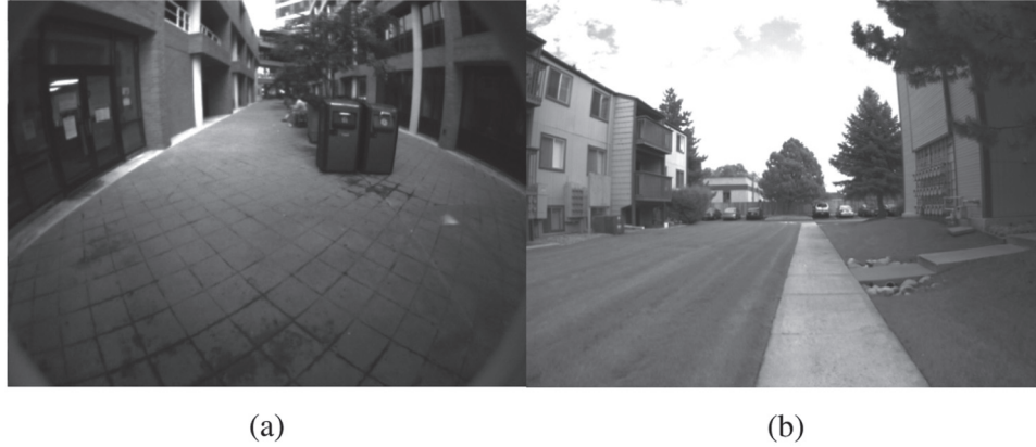
Fig. 5. Comparison of images obtained from rig A (a) and rig B (b) as described in Section 3. Rig A is a mobile hand-held device with a wide-angle lens and a global shutter camera capturing at 30 fps and with 640 \times 480 resolution. Rig B is a custom hand-held device with a global shutter camera capturing at 30 fps and with 1280 \times 960 resolution downsampled to 640 \times 480 . The picture quality and contrast of rig B is generally much better. Both rigs use a commercial grade MEMS IMUs: rig A sampled at 120 Hz and rig B at 200 Hz. Rig B features a much larger lens and higher quality camera.
